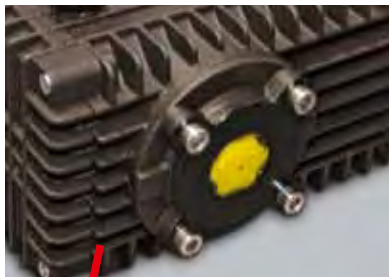
Sight glass for oil level check
